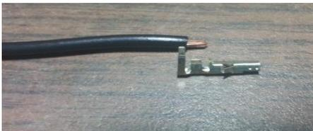
2. Insert the wire into the connector:
